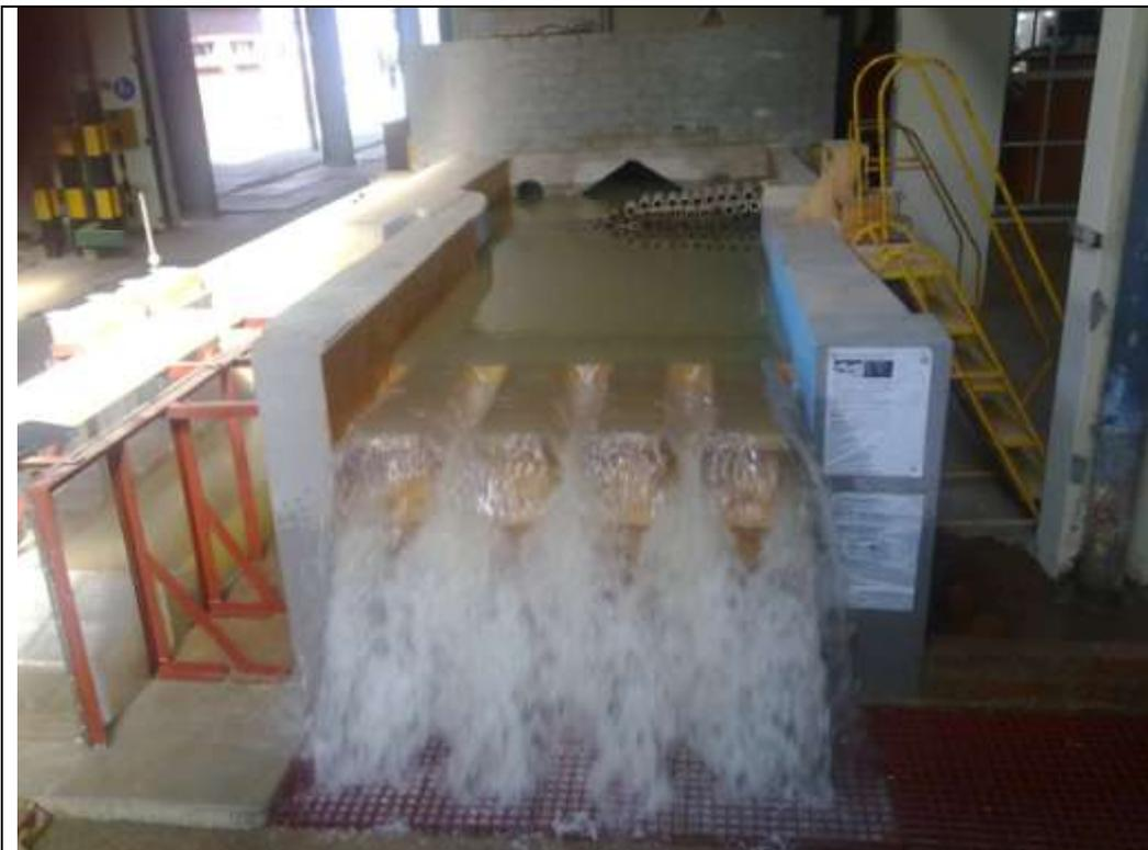
Testing of hydraulic model of PKW during extreme flood conditions (SEF).
