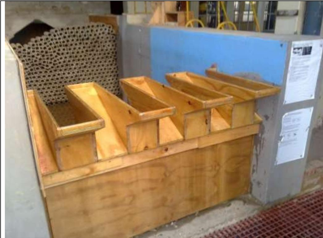
Early hydraulic model of piano key weir (PKW) to be used for 7 m raising of spillway of Hazelmere Dam.
